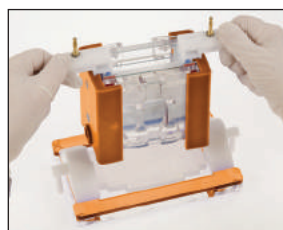
Transfer to casting base and tighten cams
