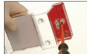
Cassette Type Electrodes can be easily replaced by the user
